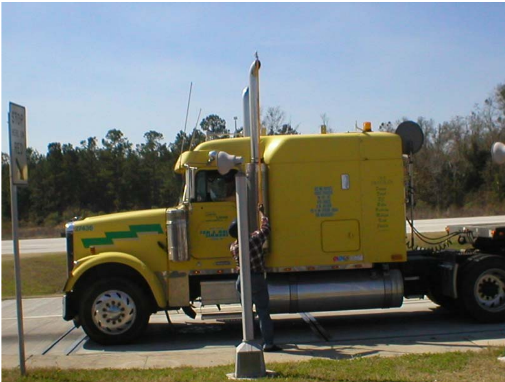
Figure B.8: Calibration of STI Vehicle Scanner – Staff Measurement of Truck Height
