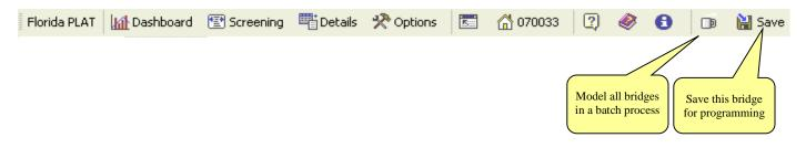
The Batch Process button loads every bridge listed on the Screening worksheet, analyzes it using the PLAT models, then saves the results in the <u>PLAT Results Database</u>. This database is a Microsoft Access file separate from your BrM database. This process can take awhile, possibly six hours or more if you analyze the entire inventory. Fortunately, this is something you would normally do only once a year.
